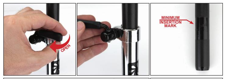
For longer distance rides raise the saddle to get a full leg extension when pedaling. For training or off-road riding you may want to lower the saddle slightly for more manueverability. Tighten quick-release style clamps with medium to firm hand pressure. Turn the tension adjusting nut clockwise while keeping the cam lever from rotating to increase clamping force or counterclockwise to decrease the clamping force; tighten bolt-on clamps to 5-6Nm. **TOOLS NEEDED:**
