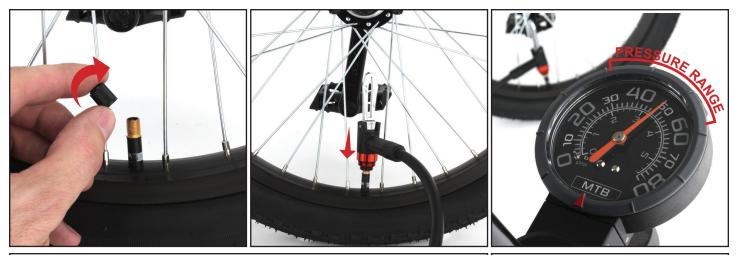
Using the air valve on the wheel and a manual air pump, inflate your tire according to your type of riding. Each tire will have maximum and minimum air pressures listed on the sidewall. Do not ride above or below the tire's rated pressures. Use higher pressures for smooth streets or longer rides and lower pressures for offroad and lower-traction surfaces.
