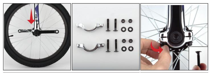
Position the wheel assembly with the right crank arm facing you. Position the unicycle with the SUN logo facing your right. Seat the wheel bearings into the frame bearing cups, then install the bearing caps onto the bottom of the unicycle frame. Tighten both left and right bearing caps evenly, also keeping caps level with the frame as you tighten. If the wheel bearings bind, loosen the bearing caps slightly until binding is gone and the wheel spins freely.
